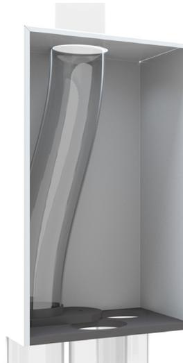
The diverter works like an exchange device that allows the carrier to reach its destination through the most direct route.
